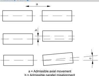
b = Admissible parallel misalignment c = Admissible angular error
