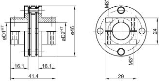
\* Maximum tightening torque: Mt = 1 Nm (plastic side)  $Mt = 1.3 \pm 10 \% Nm (metal side)$
